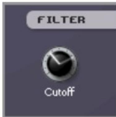
This picture shows a morphed knob state. The first value is located at eleven o'clock and morph state at two o'clock. It will result in a filter cutoff increase when using the mod wheel or MIDI velocity if assigned.
